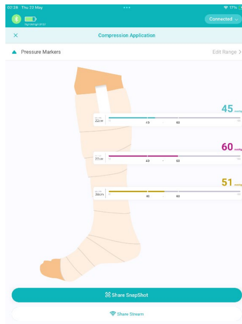
Figure 20. Example of pressures shown on “Compression Application” screen, with coloured numbers and bars indicating pressures are within range set on “Compression Application Markers” screen (grey numbers or bars represent values outside the set range).
