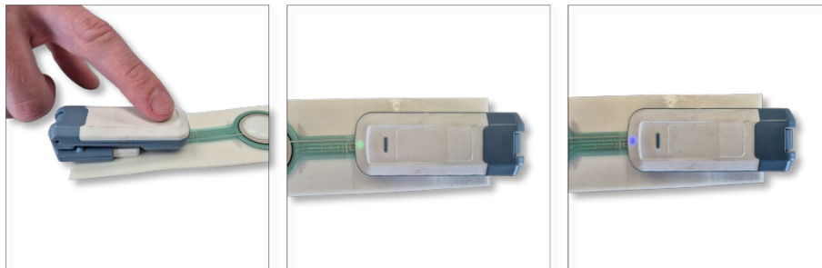
Figure 5. Switching on Transmitting Device once it has been attached to the Sensor Device, showing blue, red, and green flashing lights.
