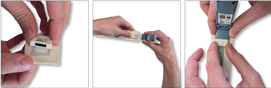
Figure 4. Attaching Transmitter Device to Sensor Device.
